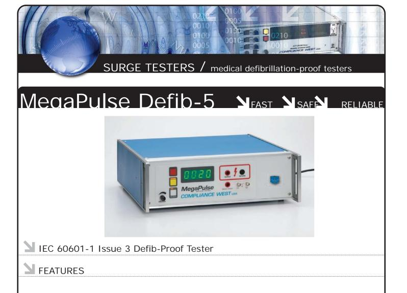
Surge Tester built to the requirements of IEC 60601-1:2005 (Issue 3) Figure 10 (IEC 60601-1 Figure 50 in older versions). Optionally can conduct IEC 60601-1:2006 Figure 11; IEC 60601-2-34; IEC 60601-2-49; IEC 60601-2-27; EC-13; and EC-53. All these tests use the same 5000V source with differences in output waveshaping. The options include the various waveshaping output circuits required for each test.
